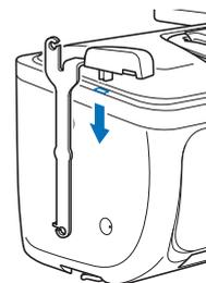
**11** Pass the yarn through the telescopic thread guide and the yarn guide (①) to (②).
