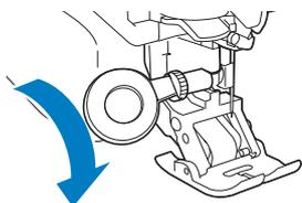
3 Place one hand on each side of the presser foot to hold the fabric secure while sewing.
