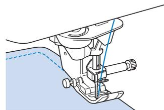
Shorten the stitch length setting to obtain a fine stitch. Sew slowly, keeping the seams parallel with the fabric edge as you guide the fabric around the curve.
