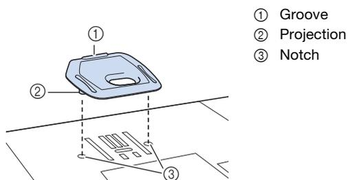
To remove the embroidery needle plate cover, place your fingernail in the groove and lift the plate out.
