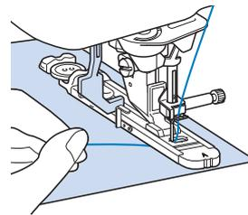
→ Once sewing is completed, the machine automatically sews reinforcement stitches, and then stops.
