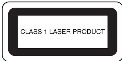
The laser beam emitted by the laser unit installed in this machine is restricted to an output at a safe level. However, the machine contains 6-milliwatt, 630-640 nanometer wavelength, 6-12 degree at parallel divergence angle, 28-40 degree at perpendicular divergence angle, InGaAlP laser diodes. Therefore, eye damage may result from disassembling or altering this machine.
