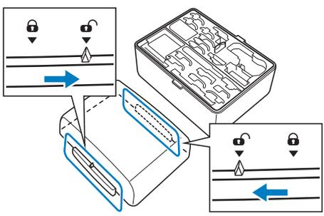
2 Place the lid on top of the case so that the notches in the lid align with the tabs on the case, and then slide the bar on each side back to the locked position.
