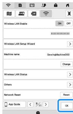
→ The name beside [Machine name] is the name that will be used when registering the machine with embroidery editing software (PE-DESIGN version 11 or later) or Design Database Transfer in order to transfer files.
