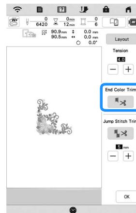
→ The key will display as
