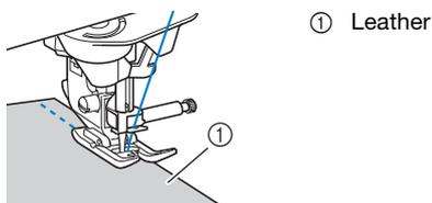
If the leather or vinyl fabric sticks to the flat bed attachment, sew with copy paper or tracing paper placed on top of the flat bed attachment so the fabric moves smoothly.
