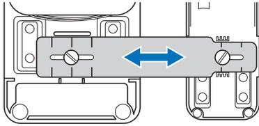
**3 Firmly tighten the mounting screws to secure the main foot controller and side pedal.**
