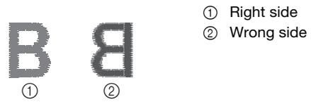
Follow the operations described below to adjust thread tension according to the situation.
