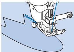
When sewing around corners, stop the machine with the needle in the fabric just outside of the appliqué, raise the presser foot lever, and then turn the fabric as needed to change the sewing direction.
