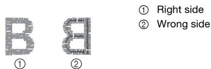
Touch **+** in **Tension** to tighten the upper thread tension. (The tension number will increase.)
