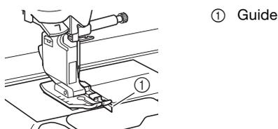
**2** Use the guide and marks on the presser foot to sew accurate seam allowances.
