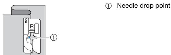
When you change the needle drop point, raise the needle, and then use  $\nabla$  and  $\wedge$  to decide the needle drop point. (The stitch width setting is in neither millimeters nor inches.)
