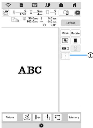
1 Switch on/off the 2-point embroidery positioning function with a LED pointer.
