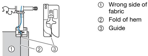
**11** Adjust the stitch width until the needle slightly catches the fold of the hem. (page 57)
