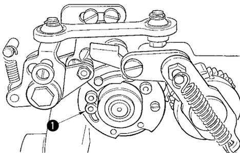
To make 8 stitches, loosen stitch number adjusting screw ❶ and fix it to the position as shown in the illustration.
