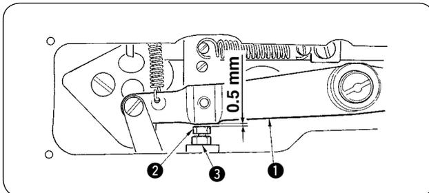
Provide a 0.5 mm clearance between the end face of button clamp lifting lever ① and adjusting screw ② at the stop-motion position (refer to "3-14 Adjusting the position of the stop-motion", p.8) and tighten with adjusting screw nut ③.
