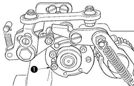
When stitch number adjusting screw ❶ being set for "8 stitches" has arrived at the left end, loosen stitch number adjusting screw ❶ and fix it to the position as shown in the illustration.
