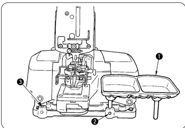
Insert the posts of button tray ① in hole on the right of the machine sub-base and tighten each setscrew ②. If it is difficult for the operator to pick up the buttons on the right side, change it to hole ③ on the left side.
