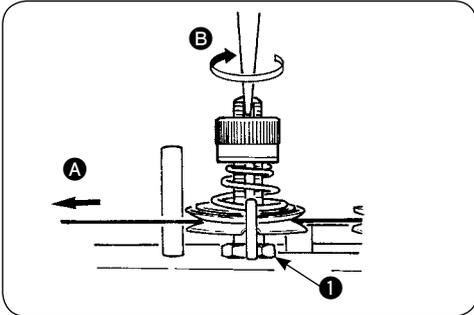
Turn the needle driving pulley as you draw the thread in the direction of arrow mark **A** and you will find a point at which the tension discs on the tension post No. 2 release the thread. At this moment, the standard distance from the top end of the needle bar bushing (upper) to the top end of the needle bar is 44 to 47 mm (in case of the needle of TQ X 7, 54 to 57 mm).
