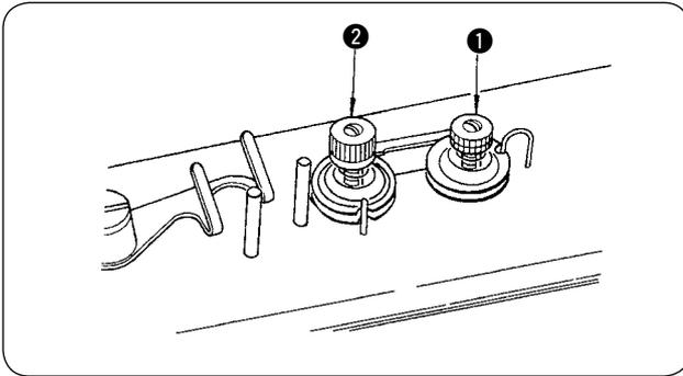
Tension post No. 1 ❶ is used to adjust the thread tension to sew on the button and a relatively low tension will be enough. Tension post No. 2 ❷ is used to adjust the thread tension applied to the root of the button sewing stitches. This tension must be determined according to the type of thread, fabric and thickness of the button and must be higher than that of tension post No. 1 ❶. Turn the tension nuts clockwise to increase or counterclockwise to reduce the thread tension.
