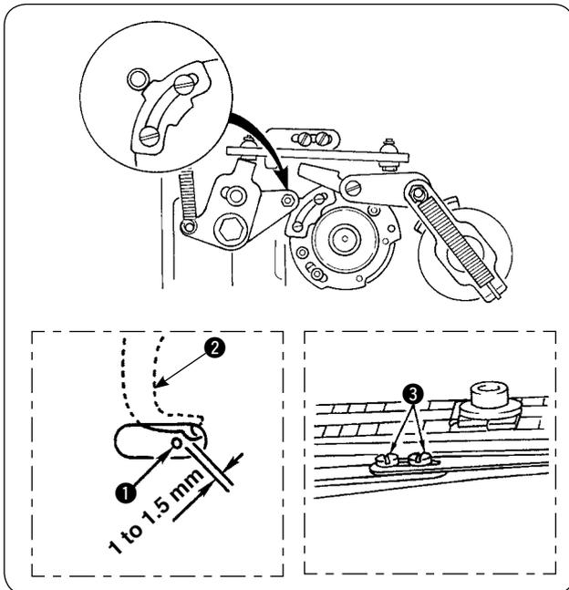
Loosen screws ❶ and adjust so that a clearance of 1 to 1.5 mm is provided between the needle ❷ and the knot tying plate ❸ when the roller of the knot-tying arm gets on the outmost periphery of the knot-tying notch.
