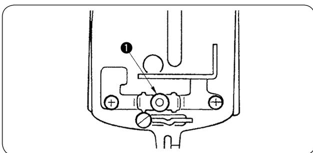
If the formation of seams at the start of sewing is failed and the seams are formed on the way even when the thread pull-off lever is adjusted, turn thumb nut ① (double nut) to decrease the thread tension.
