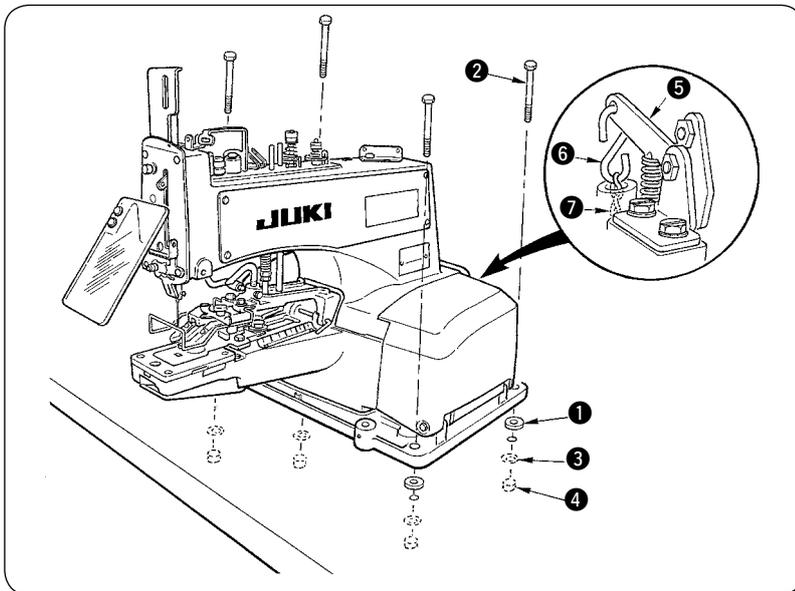
Put rubber cushion ① on the table, place the machine head on the rubber cushion and fix it to the table using screws ②, plain washers ③ and nuts ④. Attach "S" chain hook ⑥ and chain ⑦ to stop motion trip lever ⑤.
