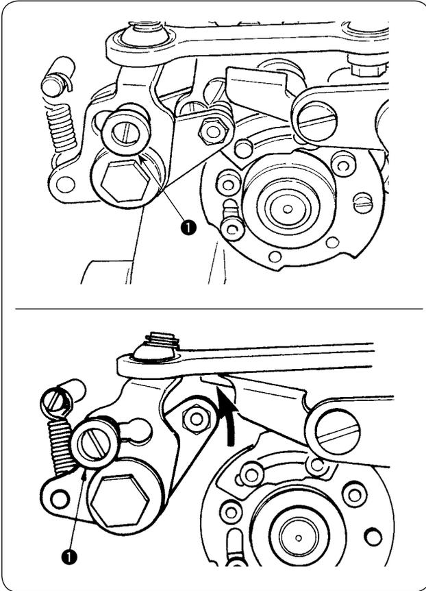
To make “with knot-tying”, pull knot-tying changeover knob ❶ toward the front and place it to the position in the figure.
