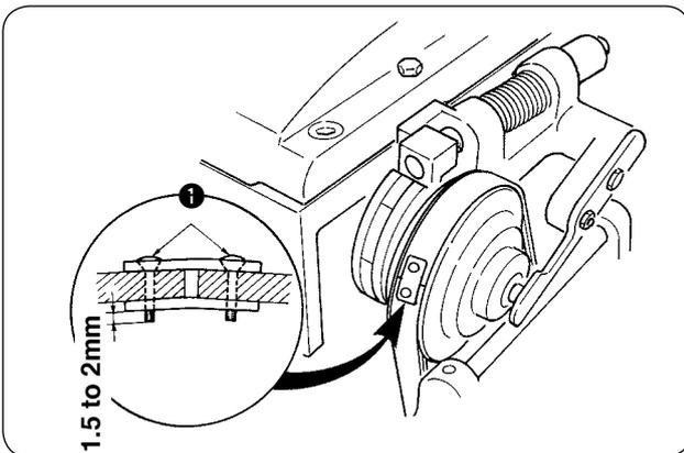
Tighten connecting screws ❶ of the belt so that the screws protrude approximately 1.5 to 2 mm from the reverse side as the standard.
