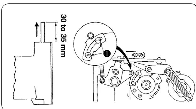
Loosen screws ❶ and adjust so that the roller of the knot-tying arm comes in contact with the knot-tying notch when the needle bar goes up at the fourteenth stitch as high as 30 to 35 mm (40 to 45 mm when a TQ x 7 needle is used) above the needle bar upper bushing.
