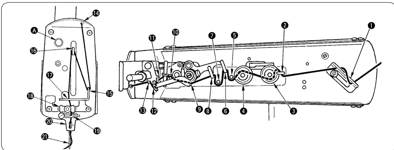
Thread the machine head in the order of ① to ②① as shown in the illustration given above. Then, pass the thread through the needle eye from the front for approximately 60 to 70 mm as you depress nipper releasing knurled thumb nut A.
