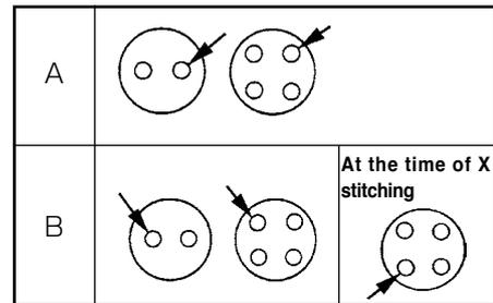
To adjust the thread pull-off lever ❶, insert a screwdriver through an opening in the machine arm side cover (left), loosen screw ❷ and adjust the position of nipper bar block (rear) ❸ to the left or the right. If the end of thread is drawn from arrow hole A in the button after sewing, change the position of nipper bar block (rear) ❸ to the left. Move the lever to the right when the thread end comes out from arrow hole B.
