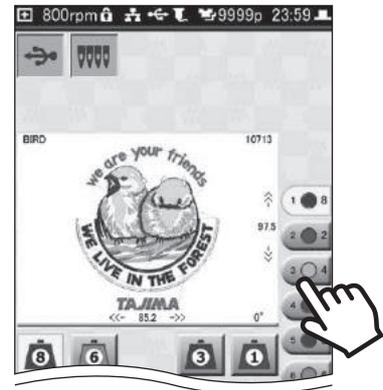
The icon of the step that was tapped and the needle No. set for the step are highlighted in yellow.
