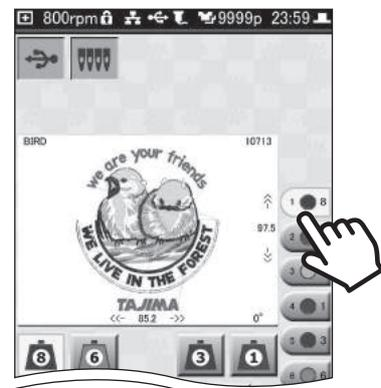
2. Tap the needle No. (1 to 8) that has the thread of the color that you want to assign to step 1.
