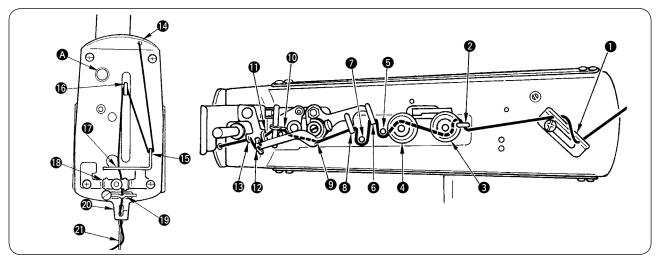
Thread the machine head in the order of **1** to **2** as shown in the illustration given above. Then, pass the thread through the needle eye from the front for approximately 60 to 70 mm as you depress nipper releasing knurled thumb nut **3**.
