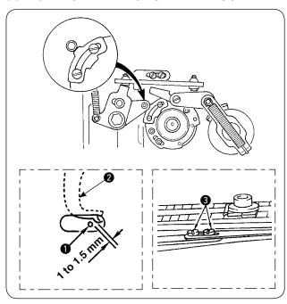
Loosen screws **1** and adjust so that a clearance of 1 to 1.5 mm is provided between the needle **2** and the knot tying plate **3** when the roller of the knottying arm gets on the outmost periphery of the knottying notch.
