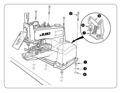
Put rubber cushion ① on the table, place the machine head on the rubber cushion and fix it to the table using screws ②, plain washers ③ and nuts ④. Attach "S" chain hook ⑥ and chain ⑦ to stop motion trip lever ⑤.
