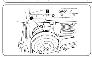
Adjust so that claw ① of the stop-motion cam comes in contact with stop-motion hook ② when the sewing machine completes the sewing and stops.
