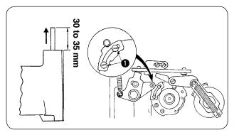
Loosen screws • and adjust so that the roller of the knot-tying arm comes in contact with the knot-tying notch when the needle bar goes up at the fourteenth stitch as high as 30 to 35 mm (40 to 45 mm when a TQ x 7 needle is used) above the needle bar upper bushing.
