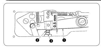
Provide a 0.5 mm clearance between the end face of button clamp lifting lever **1** and adjusting screw **2** at the stop-motion position (refer to "3-14 Adjusting the position of the stop-motion", p.8) and tighten with adjusting screw nut **3**.
