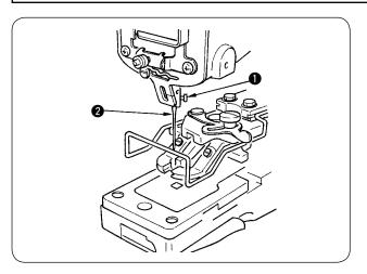
★ Use a standard needle of TQx1 #16. Loosen setscrew ① and hold needle ② with the long groove facing toward you. Then fully insert it into the hole in the needle bar, and tighten setscrew ①.
